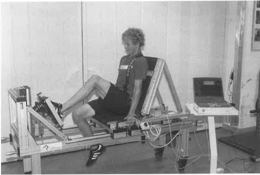
Fig. 1: Unilateral leg strength testing
